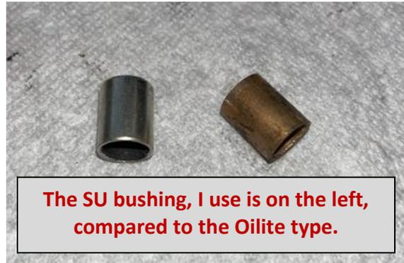
**The SU bushing, I use is on the left, compared to the Oilite type.**
